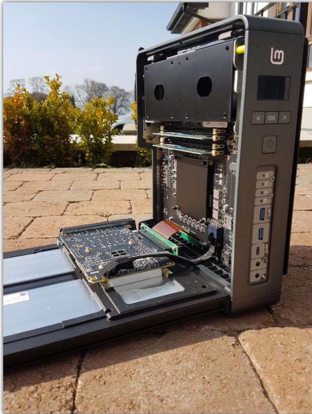
Inside the box, the components are neatly organized and easily accessible. It's very easy to get to the RAM or to pull the lever to detach the storage bay, which on top of the NVMe drive attached to the motherboard, has room for 4 additional SSDs.
