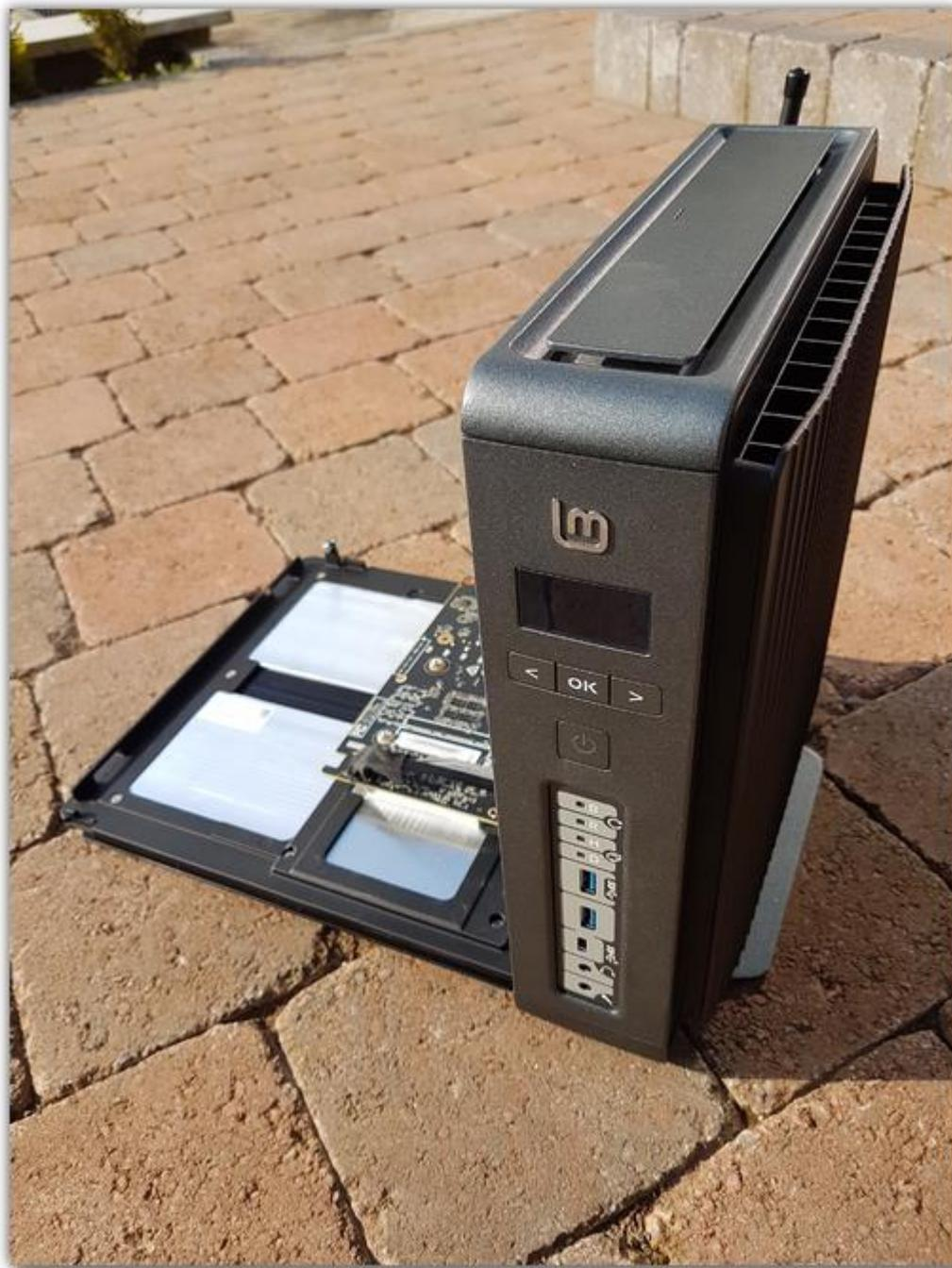
The NVIDIA graphics card is stuck against the inside of the lid to maximize its surface contact and thermal dissipation through the left heat sink.
