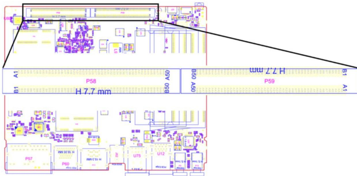
Figure 3 – B2B connector footprint view (note for 180deg offset between the connectors)
