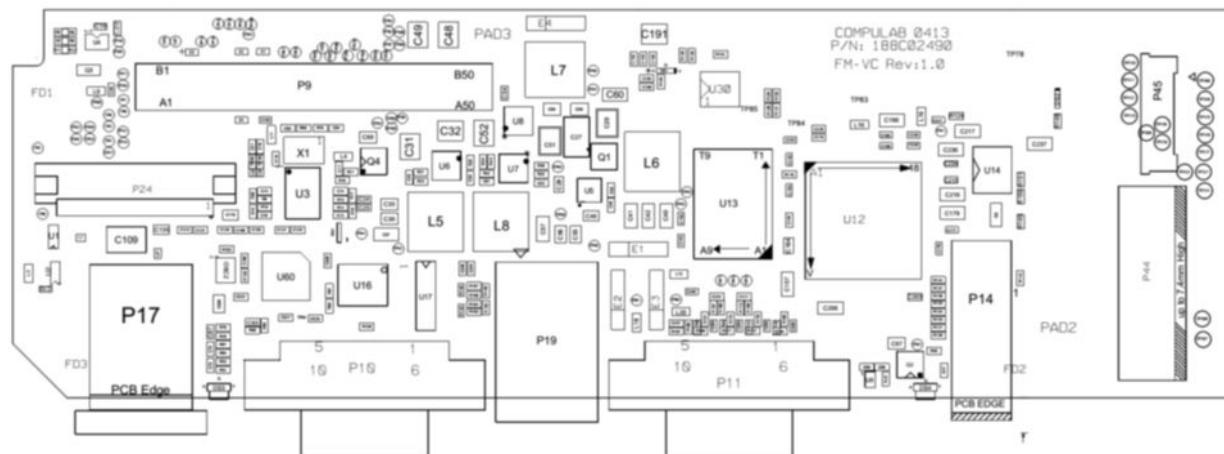
Figure 28 – FM-VC PCB Assembly Bottom
