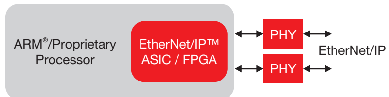
Figure 8: Integrated EtherNet/IP with processor
