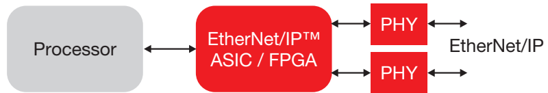
Figure 7: EtherNet/IP with ASIC and external processor
